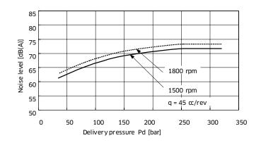
Noise level measured in an anechoic chamber where distance from microphone to pump is 1 metre. Measurement accuracy +/- 2 dB(A)
