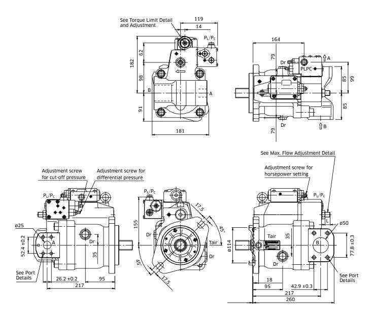
Note: for counter clockwise rotation, the suction port 'B' and the delivery port 'A' are reversed.
