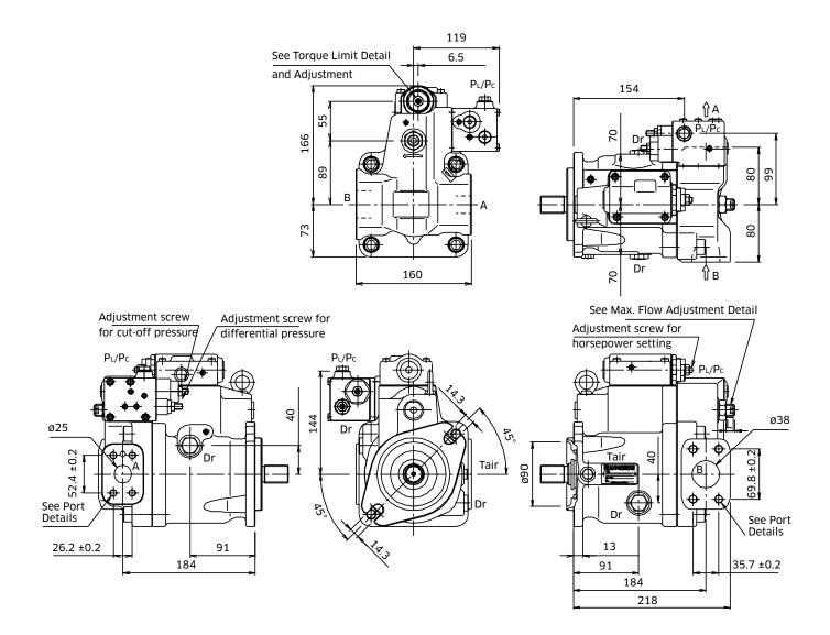
Note: for counter clockwise rotation, the inlet port 'B' and the delivery port 'A' are reversed.
