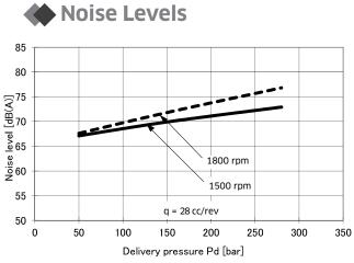
Noise level measured in an anechoic chamber where distance from microphone to pump is 1 metre. Measurement accuracy +/- 2 dB(A)
