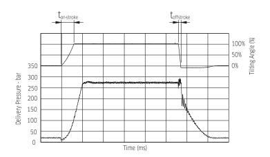
Note: The response values shown in the table above are typical of those experienced in the laboratory. Actual reposnse time will vary with different hydraulic circuits.
