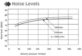
Noise level measured in an anechoic chamber where distance from microphone to pump is 1 metre. Measurement accuracy +/- 2 dB(A)
