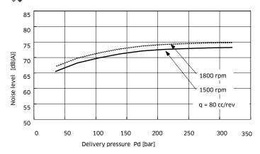
Noise level measured in an anechoic chamber where distance from microphone to pump is 1 metre. Measurement accuracy +/- 2 dB(A)
